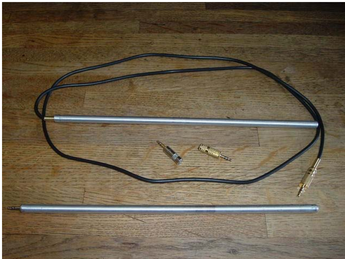
Figure XXIII. Measurement Microphones Used in Distortion Analysis
