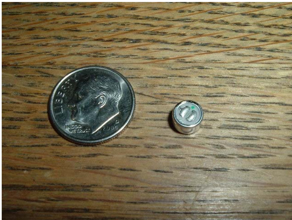
Figure XVII. The Panasonic WM61A Electret Cartridge and a Dime
