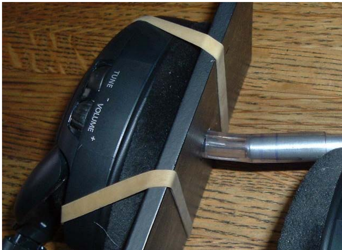
Figure XXXI. Headphone Response Measurement Using the WM61A as a Measurement Microphone
