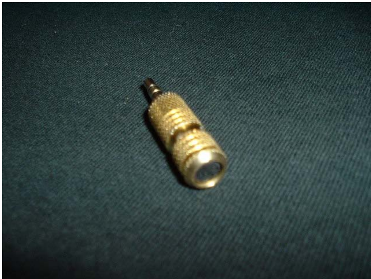
Figure XXI. The Finished Measurement Microphone Using the Panasonic WM61A Electret Cartridge
