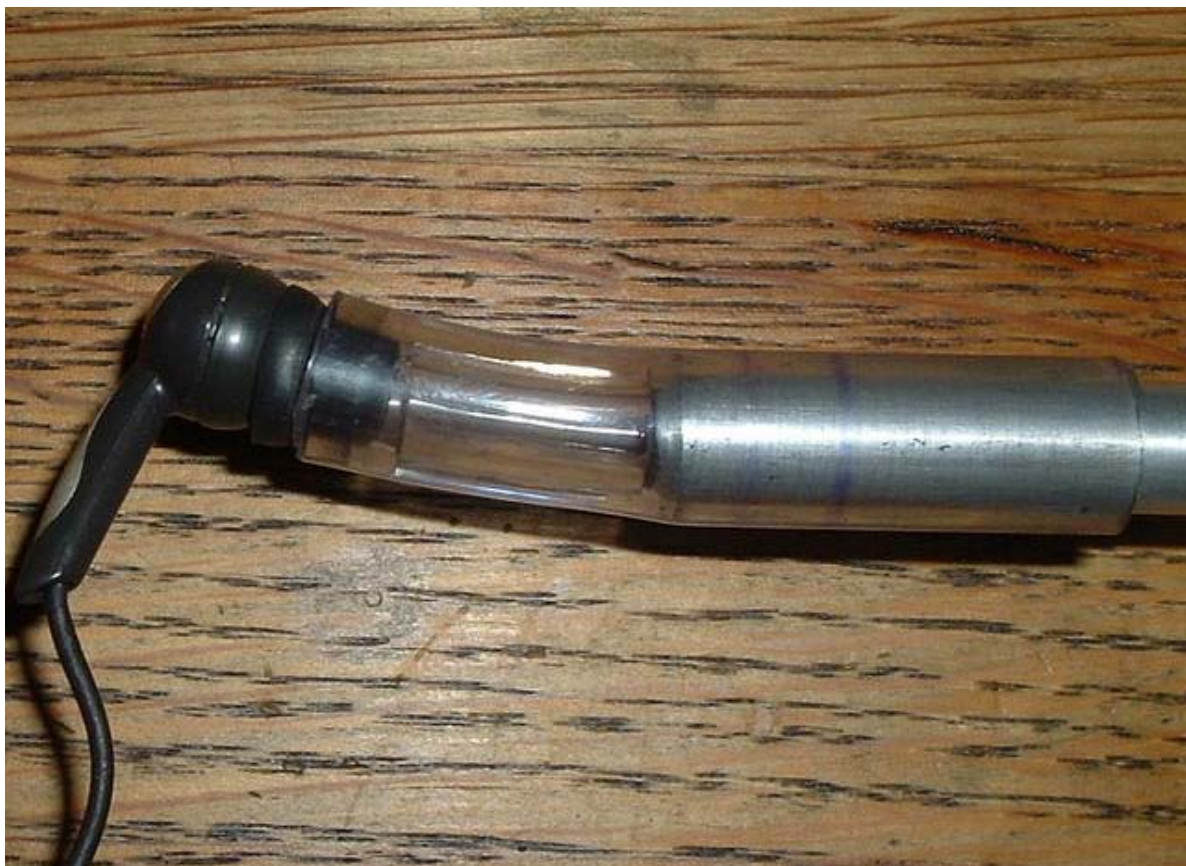
Figure XXXIV. Earbud Response Measurement Using the WM61A as a Measurement Microphone
