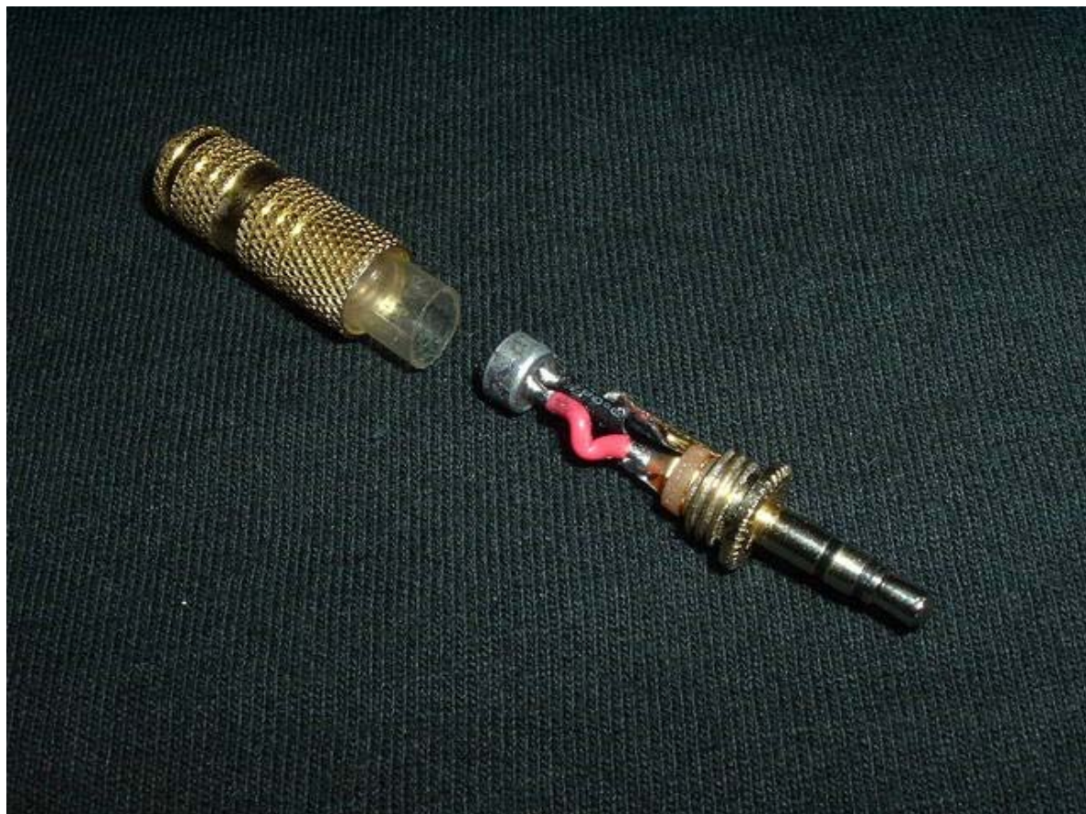
Figure XX. The Panasonic WM61A Electret Cartridge and Housing
