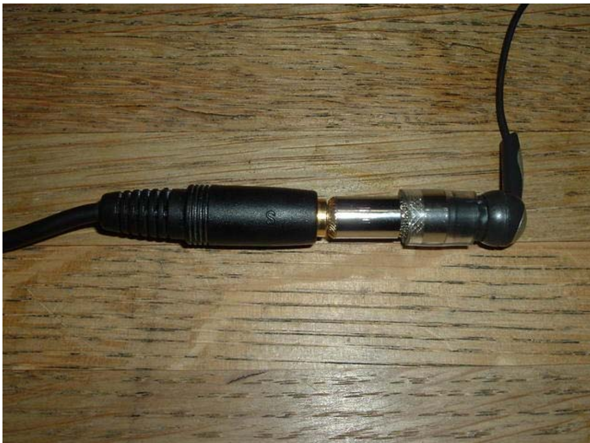
Figure XXII. Calibrating the Measurement Microphone Using the Panasonic WM61A Electret Cartridge
